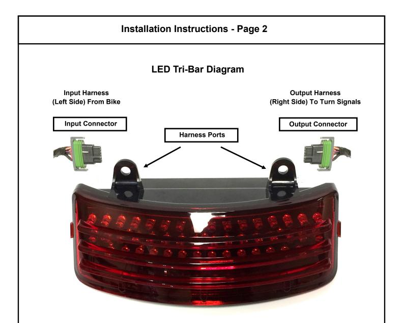
Plug the harness connectors into the new Tri-Bar, noting the rectangular ports on the back side of the unit. Left side should be going to the bike, the right side is the output to the turn signals. Make sure that the connector orientation is correct going into the ports, they are keyed one way, if the connector does not want to snap in, flip it around and try it again.
